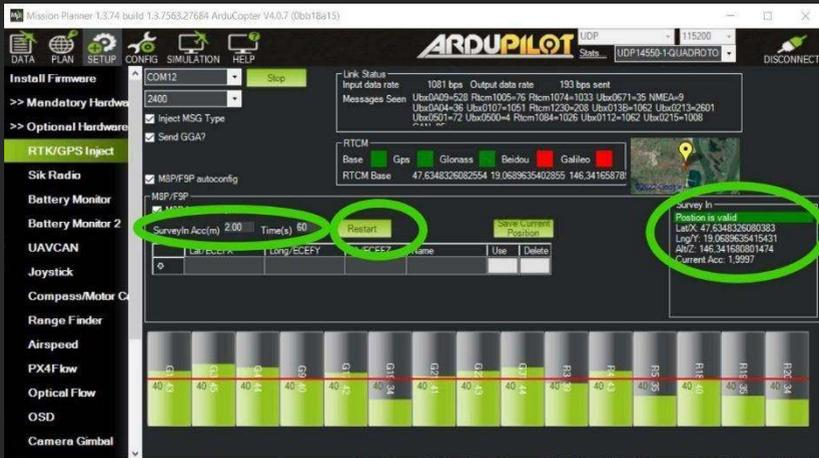
7: The interface displays the number of satellites and the detected signal strength with columns. If the expected values are already within the defined absolute accuracy, the **Position is valid** message is shown on the right, marked in green. Depending on the conditions (e.g. weather, humidity), reaching the absolute accuracy can vary significantly, experience shows that for 2m at least a few minutes and for 30cm about 1 hour may be required even under ideal conditions.
