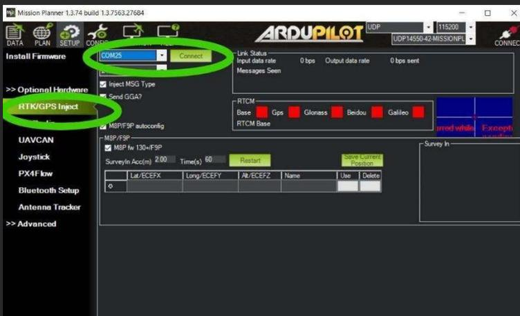
5: The **SurveyIn Acc(m)** field is used to set absolute geographic accuracy that you expect, the **Time(s)** field is the minimum survey time you expect.
